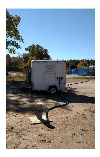
The pump test for the proposed extraction well which will help to control the 1,4-dioxane plume associated with the Nuclear Metals Incorporated Superfund site, was conducted in the fall of 2016. Water was stored in temporary tanks at our 16 Knox Trail property and disposed of at a proper treatment facility.
